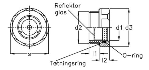
$\begin{array}{lll} d1 & = 14 \\ d2 & = M20x1,5 \\ d3 & = 26 \\ l1 & = 8.5 \\ l2 & = 7.5 \\ Max \ pressure = 25 \ Bar \\ s & = 23 \end{array}$
